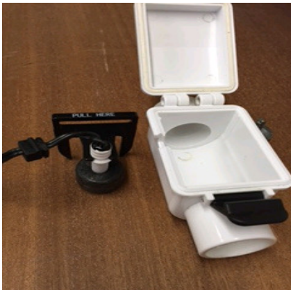
REMOVE FLOAT SWITCH (SWITCH CAN BE ADJUSTED UP/DOWN)
