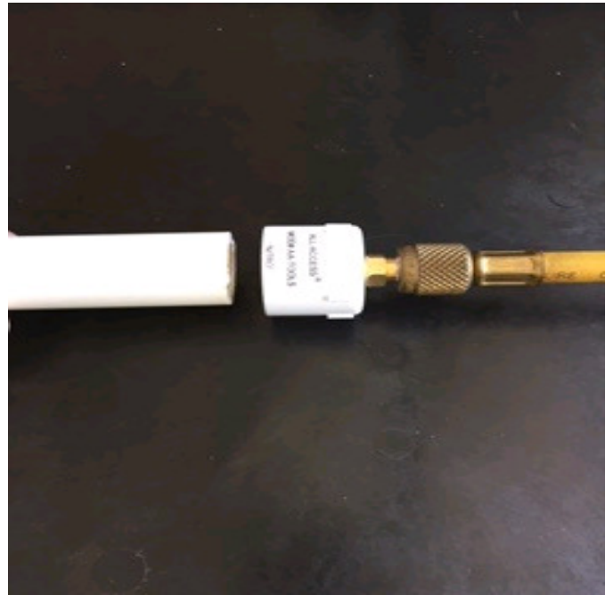
NITROGEN TOOL ON ¾” PVC
