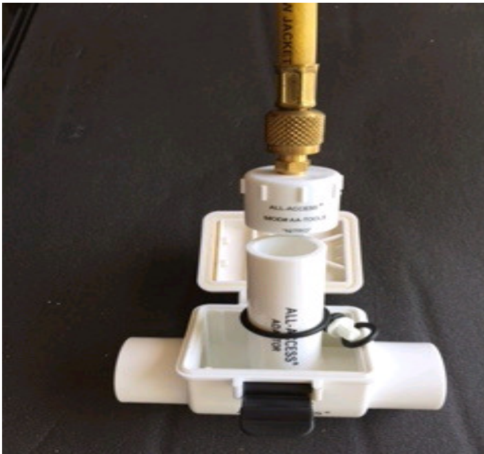
NITROGEN TOOL ON ADAPTOR
